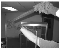
4. Install H-channels on top of main shields. Outside edge of H-channel should line up with outside edge of shield below.
