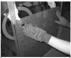
**14.** Place S2 and S1 baffles in position on shields. Have assistant apply opposing pressure from opposite side then press baffle corners to secure Velcro to shield.
