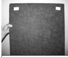
**13.** Place Velcro on all four corners of S2 and S1 baffles about 1-inch from corners and peel off paper to expose adhesive.
