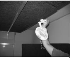
**16.** Clip fan to back of STC or top of S5-2 to aid in air exchange.
