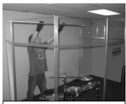
10. Adjust Lid support bar to width between end panels and rest support bar J-hooks at least 4inches from edge of end shields. Do not extend bar beyond red limit marker. Lid systems wider than 6' should use two support bars.
