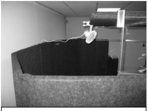
**17.** Leave a small opening in upper back of IsoPac to allow for some air exchange. If necessary, overlap S5-2 and end shields to decrease opening.
