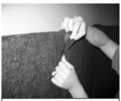
15. If included, move the S5-2 baffles into position behind kit. Use the Velcro flaps on outside top and bottom sides of S5-2s to attach S5-2 units together. Ends of baffles should overlap inside of shields or butt up against them.
